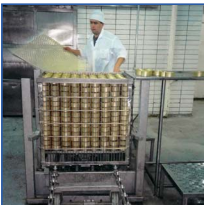
Packfix: Fleischprodukte in Aluminiumschalen Cage bottom lift: Meat products in Al-trays
